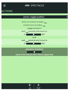
This action moves the motor between two positions, one motion on each trigger event.
