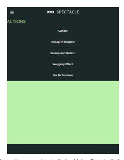
There are four actions associated with the Motion Board, all of which should be used with a single trigger pulse type input signal.
