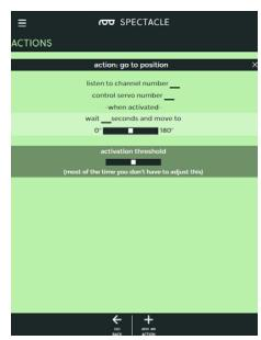
Move the servo motor from where ever it currently is to this new location after some delay.
