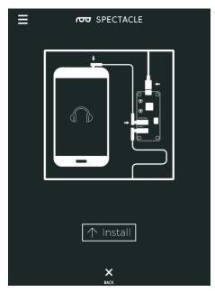
Make sure the volume on your device is turned all the way up, and that no other audio source (music, video, etc) is playing in the background. Then press and hold the "RST" button on the Director Board, press and hold the "PROG" button, then release the "RST" button.
