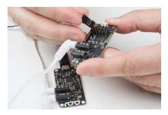
Finally, plug the Micro B end of the USB cable into the Director Board, and the other end into the wall adapter. Plug the adapter into the wall. You should see one solid light and one blinking light on the Motion Board. On the Director Board, you'll see one solid light and one light which blinks one time, then pauses, then repeats. This shows that power is present and the boards are up and running.
