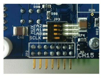
Figure 13. DIP Switch Set to All Zeros (0x20)
