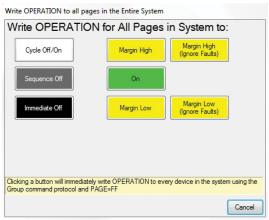
A look at the telemetry window shows the effect of the margin high or margin low operation. The following screen shot shows all rails going from nominal setpoints to margin high, margin low, and back to nominal voltages.
