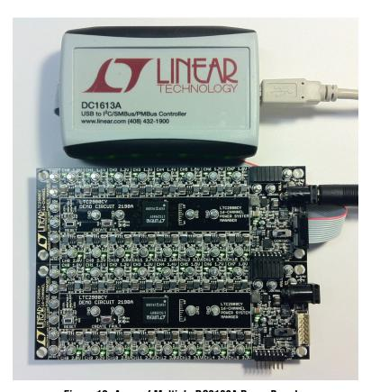
Figure 12. Array of Multiple DC2198A Demo Boards
