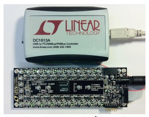
Figure 2. Connecting DC2198A Board and the DC1613 I<sup>2</sup>C/SMBus/PMBus Controller
