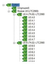
**Note**: For multiple board arrays, the GUI automatically ensures each device has a unique address. In this scenario, it is recommended at this point to store these addresses to NVM (EEPROM) by clicking the "RAM -> NVM" icon in the toolbar.
