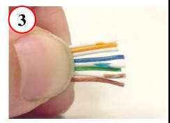
Position Wires into Correct Configuration (586-B Shown)
