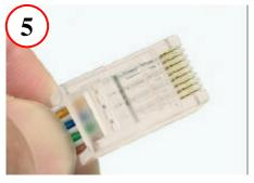
**Insert Wires Along Plug Top, Maintaining Correct Alignment**
