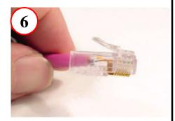
Inspect The Plug; Wires Should Be Visible from Plug Front
