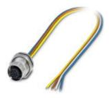
Bus system flush-type socket, PROFINET, 4-pos., M12 SPEEDCON, D-coded, front/screw mounting with Pg9 thread, with 0.5 m TPE litz wire,  $4 \times 0.34$  mm<sup>2</sup>
