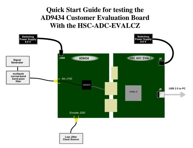
Figure 1: AD9434 ADC Evaluation Board – HSC ADC EVALC Data Capture Board
