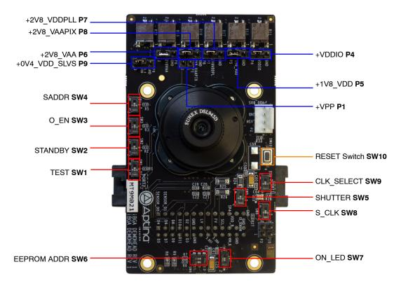
Figure 3. Top View of Evaluation Board – Default Jumpers
