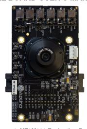
Figure 1. MT9M021 Evaluation Board
