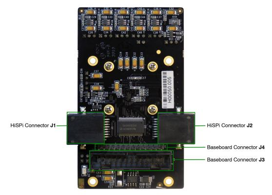
Figure 4. Bottom View of the Evaluation Board - Connector
