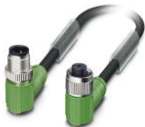
Sensor/actuator cable, 4-position, Variable cable type, shielded, Plug angled M12, A-coded, on Socket angled M12, A-coded, cable length: Free input (0.2 ... 40.0 m)
