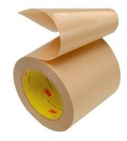
3M™ ECATT 9703 is a pressure sensitive adhesive (PSA) transfer tape with anisotropic electrical conductivity. PSA matrix is filled with silver particles enabling interconnections through adhesive thickness (the Z-axis) between substrates.
