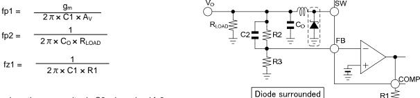
Also, by inserting a capacitor in C2, phase lead fz2 can be added.
