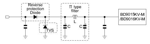
Figure 41. Filter circuit
