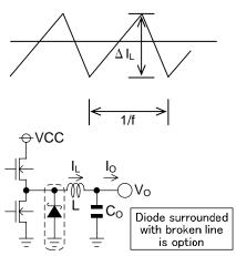
The coil value significantly influences the output ripple current. As shown in the following equation, the larger the coil, and the higher the switching frequency, the lower the ripple current.
