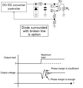
Figure 31. Measurement of Frequency Characteristic
