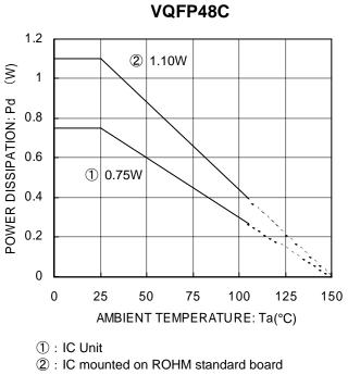
(Glass epoxy board of 70mm × 70mm × 1.6mm)
