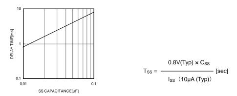
Figure 23. Capacitance vs. Soft Start Time
