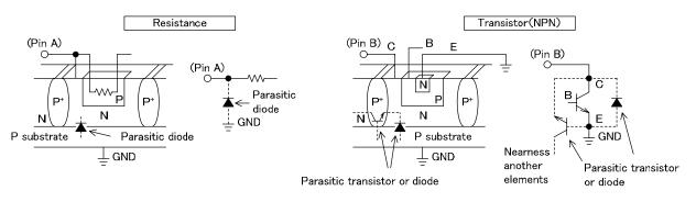
The structure example of the IC
