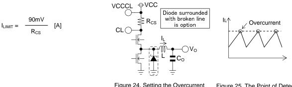
Figure 24. Setting the Overcurrent Detection Value Figure 25. The Point of Detecting Overcurrent
