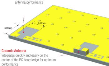
Reference PCB layout of the 2.4GHz SMT Ceramic Antenna (Refer to AS-203006-001 for more information)
