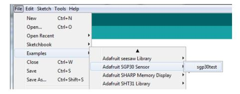
Then open up the serial console at 9600 baud, you'll see the **serial number** printed out - this is a unique 48-bit number burned into each chip. Since you may want to do per-chip calibration, this can help keep your calibration detail separate
