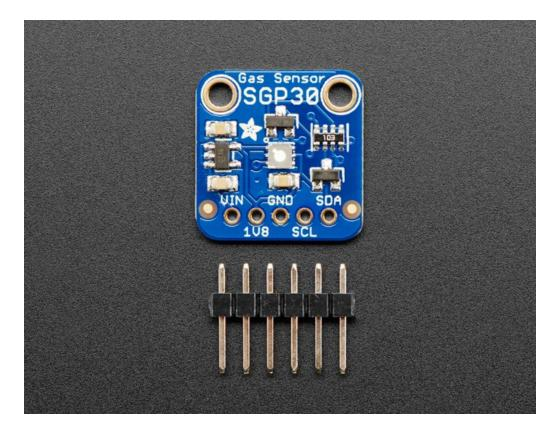
The SGP30 has a 'standard' hot-plate MOX sensor, as well as a small microcontroller that controls power to the plate, reads the analog voltage, tracks the baseline calibration, calcluates TVOC and eCO2 values, and provides an I2C interface to read from. Unlike the CCS811, this sensor does not require I2C clock stretching.
