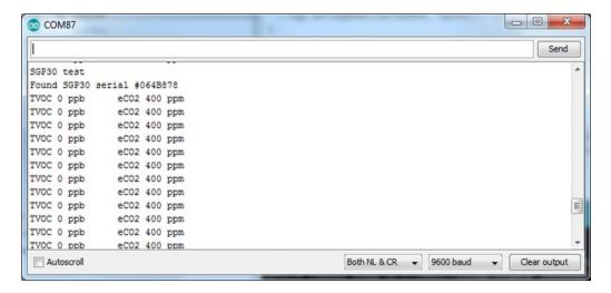
The first 10-20 readings will always be TVOC 0 ppb eCO2 400 ppm. That's because the sensor is warming up, so it will have 'null' readings.
