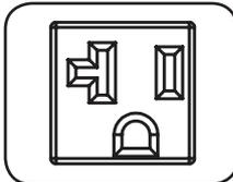
**NEMA 5-15/20R Outlets:** The outlets are color-coded to correspond with each of the independent power circuits.
