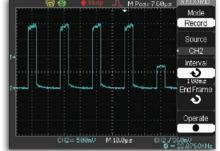
Capture and replay a sequence of up to 2500 waveforms to isolate that runt or glitch which is causing problems in your system.
