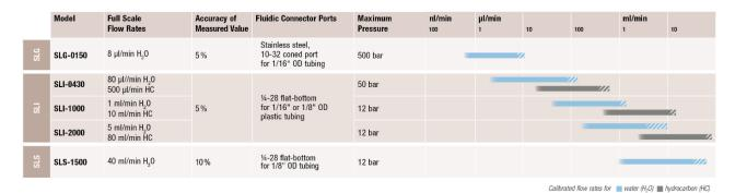
Figure 1: Sensors and their performance characteristics.
